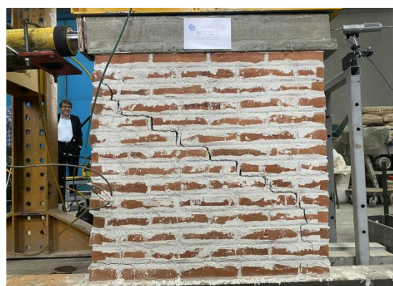
Figure 10. Shear strength - wall after testing.
