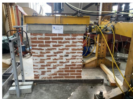
Figure 9. Testing of shear strength of masonry.
