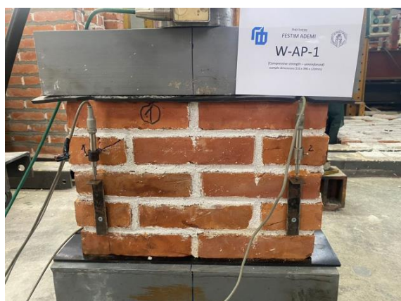
Figure 7. Testing the compressive strength of masonry.
