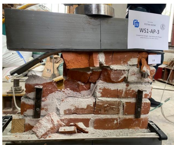
Figure 8. Compressive strength - a wall after testing (under the effect of compressive force).
