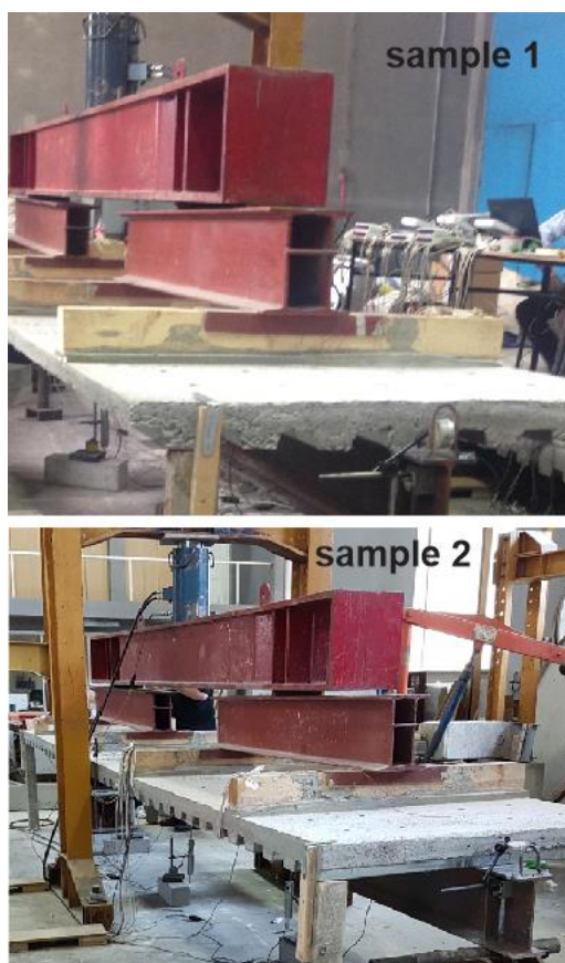
Figure 5. Test beams and load application equipment
