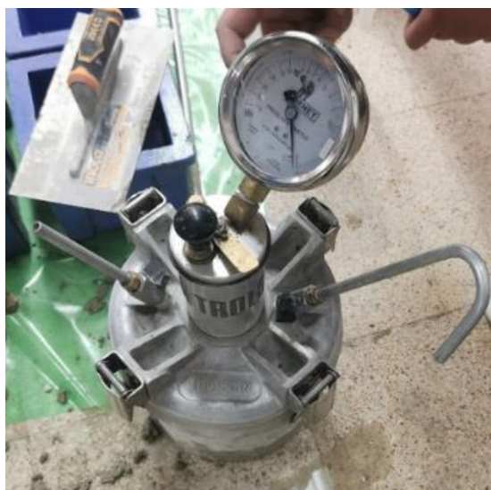
Figure 5. Pore content testing
