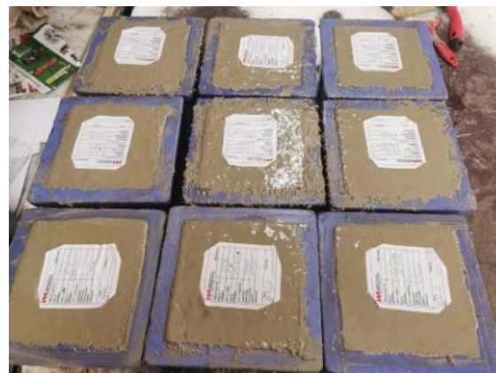
Figure 3. Fresh concrete samples for testing compressive strength
