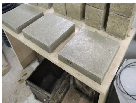
Figure 3. Fresh concrete samples for testing thermal conductivity
