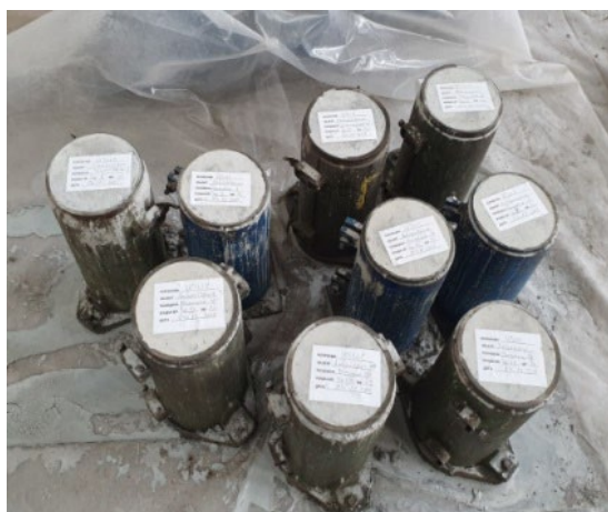
Figure 5. Photos of taken trial concrete specimens (cylinders)
