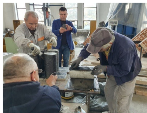
Figure 6. Preparation of strain gauges on concrete cylinders.
