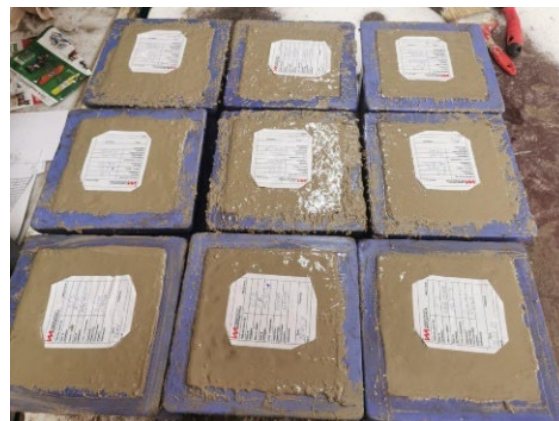
Figure 3. Fresh concrete samples for testing compressive strength
