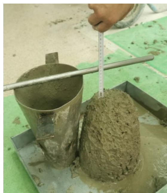
Figure 4. Consistency (slump) test
