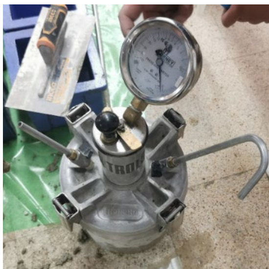
Figure 5. Pore content testing
