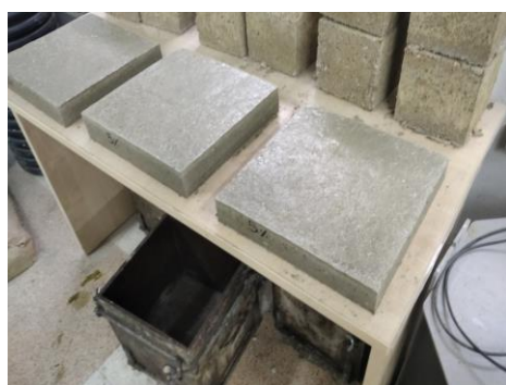
Figure 3. Fresh concrete samples for testing thermal conductivity
