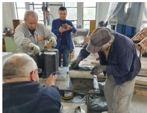
Figure 6. Preparation of strain gauges on concrete cylinders.
