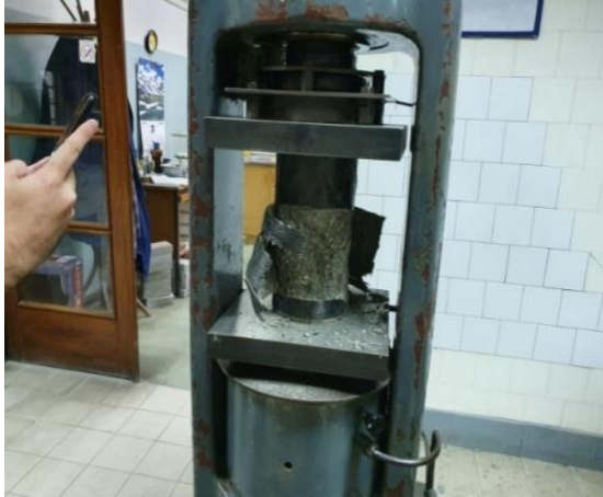
Figure 7. Testing of compressive strength of concrete wrapped with two CFRP layers- the 2 nd series.
