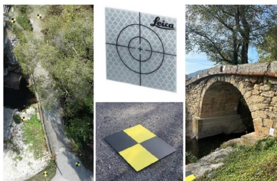
Figure 1 Figure 5. Ground control points used in field measurements
