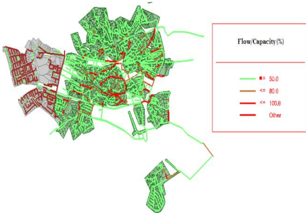
Figure 9. Flow/Capacity of the sewer system
