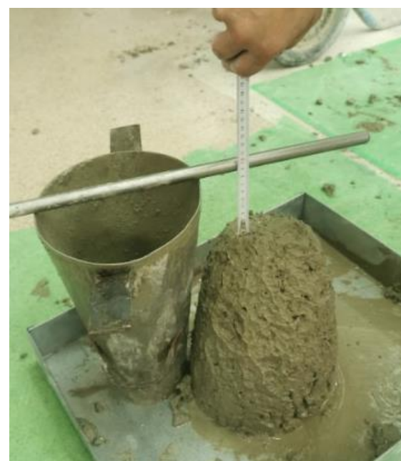
Figure 4. Consistency (slump) test
