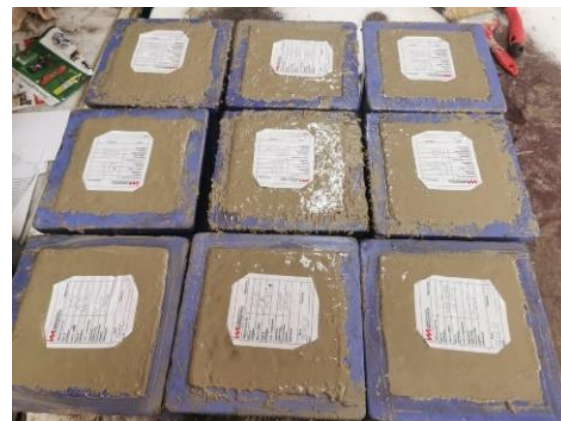
Figure 3. Fresh concrete samples for testing compressive strength
