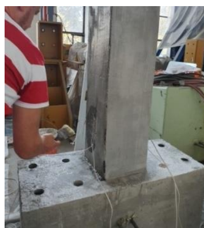
Figure 2b. Construction of the column models for experimental tests and instrumentation
