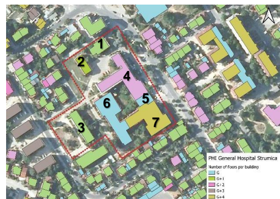
Figure 7. Existing Building Taxonomies in PHI “General Hospital” Strumica using QGIS classified by the number of floors above ground
