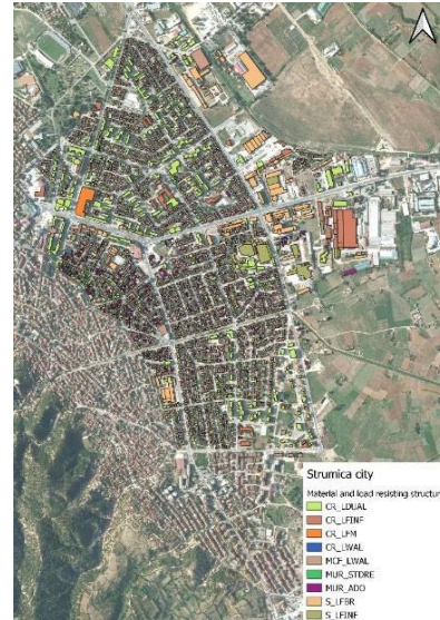
Figure 4 Existing Building Taxonomies in Strumica Using QGIS classified by material and load-resisting structure
