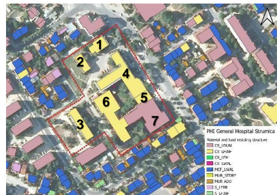
Figure 6. Existing Building Taxonomies in PHI “General Hospital” Strumica using QGIS classified by material and load-resisting structure
