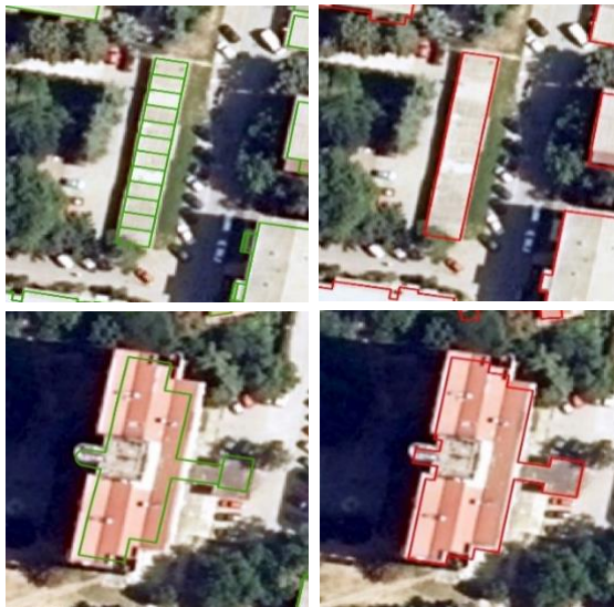
Figure 3. Building footprints registered in the cadastral system (left – green polygons), extracted building footprints based on LiDAR data (right – red polygons)
