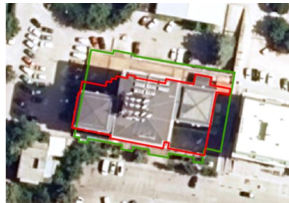
Figure 13. Building footprint registered in the cadastral system (green polygon), extracted building footprint based on LiDAR data (red polygon)
