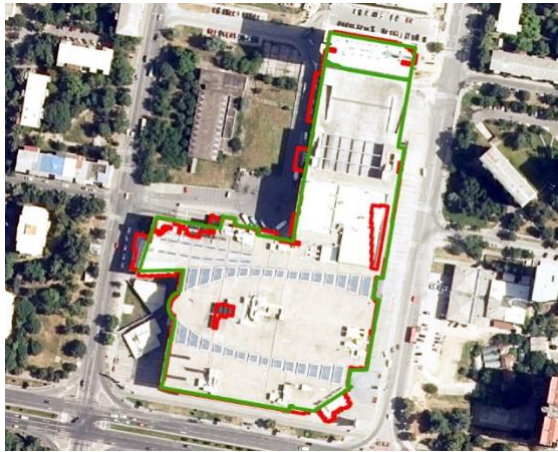
Figure 10. Building footprint registered in the cadastral system (green polygon), extracted building footprint based on LiDAR data (red polygon) – Skopje City Mall
