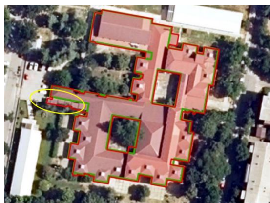
Figure 8. Building footprint registered in the cadastral system (green polygon), extracted building footprint based on LiDAR data (red polygon)
