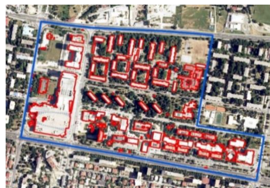
Figure 2. Extracted buildings footprints in the research area (red polygons)
