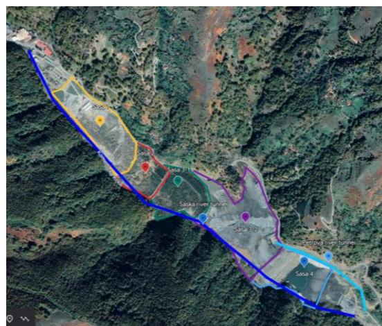
Figure 1. Layout configuration of all five TSFs in the zinc and lead mining complex 'Sasa'. The diversion tunnel for Saska river is under the right bank, whereas the tunnel for Petrova river is under the left bank. Source: Google Earth
