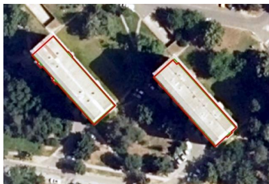
Figure 6. Building footprints registered in the cadastral system (green polygon), extracted building footprints based on LiDAR data (red polygon)
