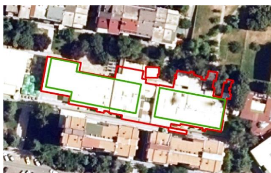
Figure 17. Building footprints registered in the cadastral system (green polygon), extracted building footprint based on LiDAR data (red polygon)
