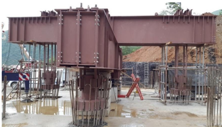
Figure 5. View of the cross beam reactive platform system during testing
