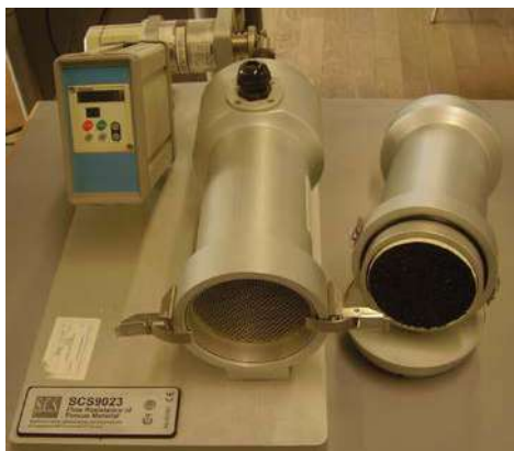
Figure 2. Airflow resistivity measuring device SCS9023
