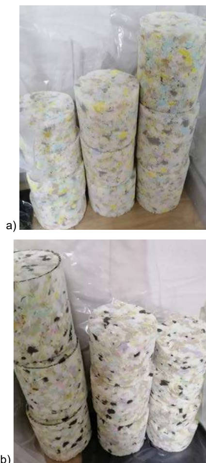
Figure 1. Rebanded polyurethane foam specimens: a) \rho=40 \text{ kg/m}^3 , b) \rho=60 \text{ kg/m}^3
