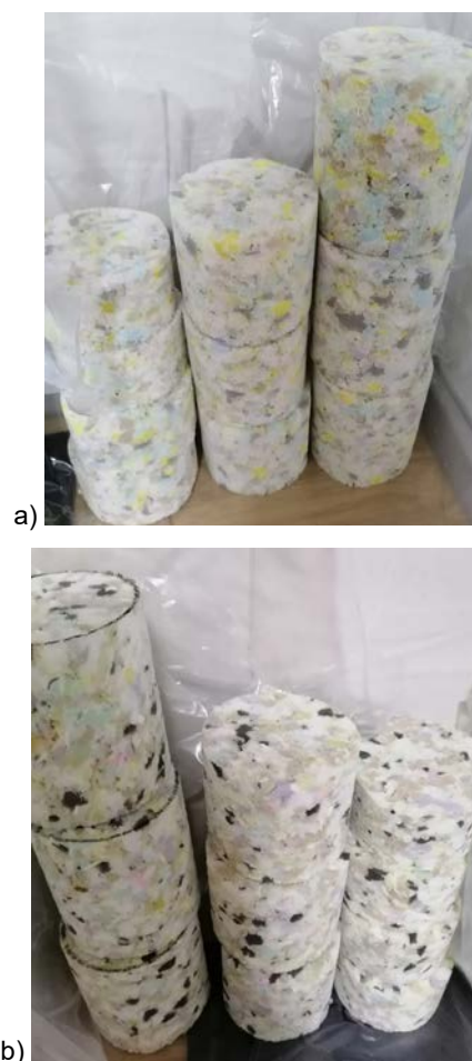
Figure 1. Rebonded polyurethane foam specimens: a) \rho=40 \text{ kg/m}^3 , b) \rho=60 \text{ kg/m}^3
