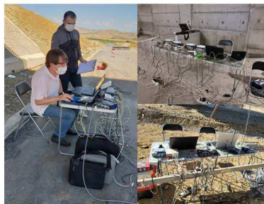
Measurements of strains and deflections during the proof loading tests of concrete bridges
