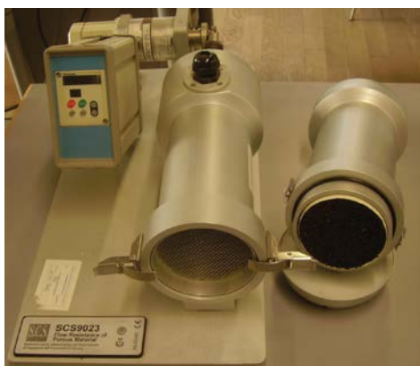
Figure 2. Airflow resistivity measuring device SCS9023
