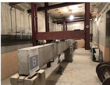
Time-dependent behavior of rc elements under sustained loads with various intensity, Laboratory for concrete and structures, FCE-Skopje
