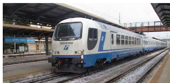
Figure 4. Mermec measuring vehicle
