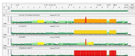
Figure 8. Performance indicators for the section Slavonski Brod-Velika Kopanica (left pavement, right lane)
