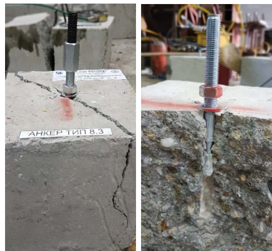
Figure 16. Failure of anchor type 7 and 8
