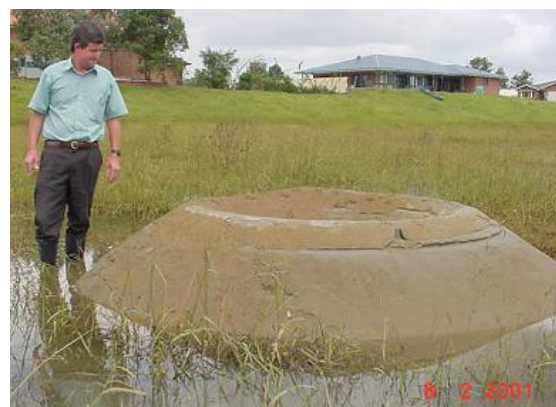
Figure 8. Boiling "volcanoes" after the flood. Retrogressive internal erosion towards the dyke causes stability loss in the long-term (photo: L. Nagy)
