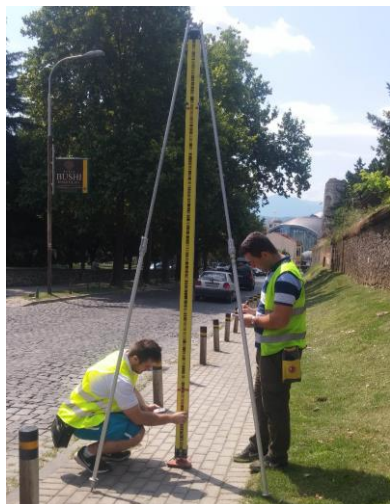
Figure 9. Measuring the temperature of the Invar rod
