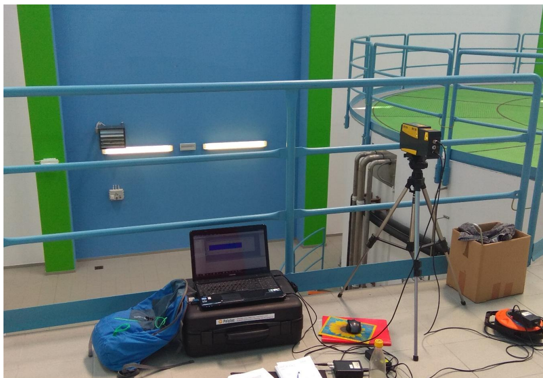
Figure 2: Example of a measurement with the Laser Doppler Vibrometer
