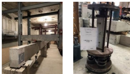
Figure 2. Test setup of RC test beams (left) and test setup for creep (right)
