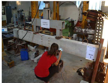
Long-term experiments on reinforced concrete elements subjected to real load histories, Laboratory for concrete and structures, FCE-Skopje
