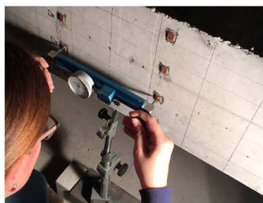
Long-term experiments on reinforced concrete elements strengthened by carbon strips, Laboratory for concrete and structures, FCE-Skopje
