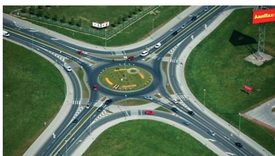
Figure 8. Classic single-lane roundabout with bypass lanes for right turns near the city of Varaždin [26]
