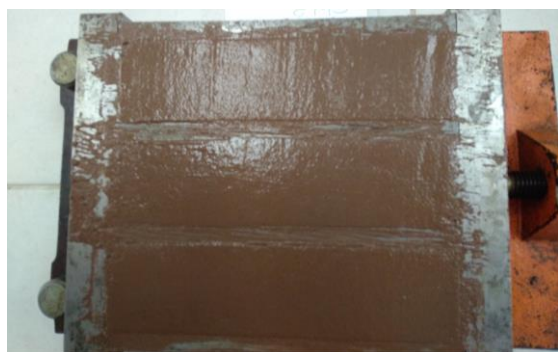
Figure 3. Mixture of mortar with high percentage of red mud (20%)
