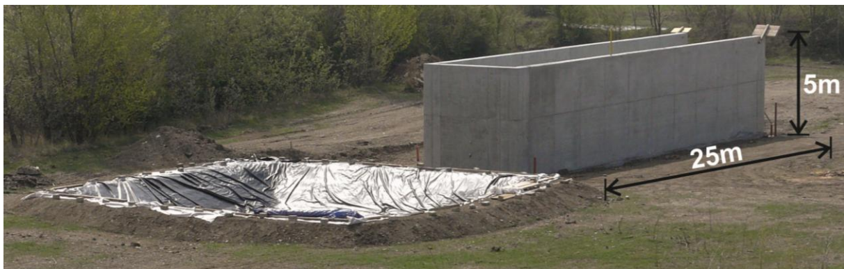
Figure 22. The large scale test facility (length 25 m, height 5 m und width 4 m) for investigating the underseepage of dykes and levees in a 1:1 scale
