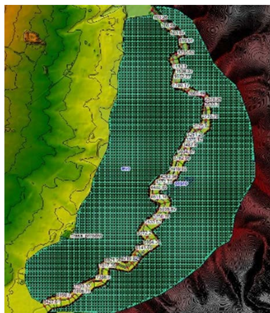
Figure 9. Calculation zone of 1D/2D hydraulic model of the river Vardar
