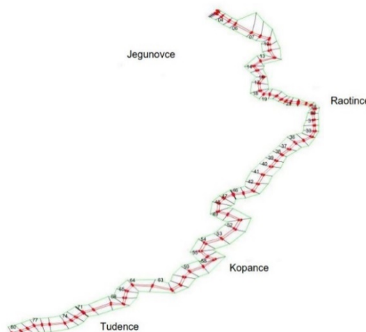
Figure 8. Situation with cross sections of 1D modelling
